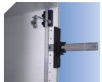
Drilling for placing invisible hinges.
