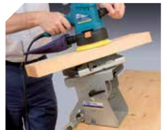
Adjustable tilting and swivelling support.
