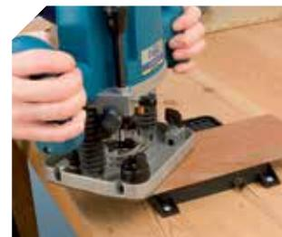
Holding small pieces on a section of the suction plate.
