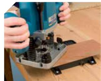
Holding small pieces on a section of the suction plate.
