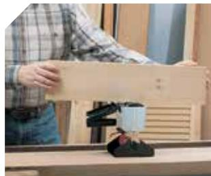
Gluing with the upper roller.
