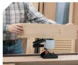
Gluing with the upper roller.
