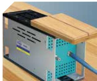
Small piece clamped on divisible suction plate.
