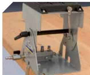
Distributor for connection of up to four auxiliary SVN470 or SVN250 units.
