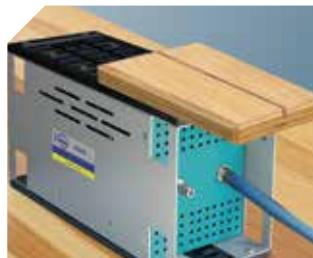
Small piece clamped on divisible suction plate.
