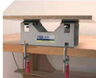
It can be fixed to the workbench by means of the two clamp screws included as standard equipment.
