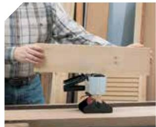
Gluing with the upper roller.
