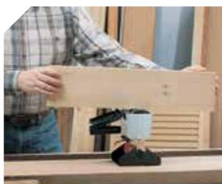
Gluing with the upper roller.
