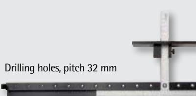
Drilling holes, pitch 32 mm
