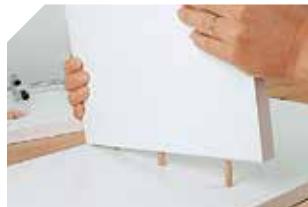
This highly practical accessory makes joints quick and easy to perform with no time lost marking reference points.
