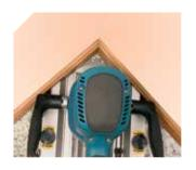
Thanks to the possibility to take away the front part of the head it is possible to arrive to the corner when cutting the skirtings.
